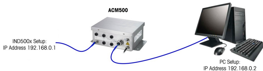
Figure 132: Example: IP Address Configuration (Crossover or Hub Configuration)
