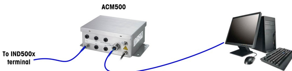
Figure 130: Connection with Crossover Cable
