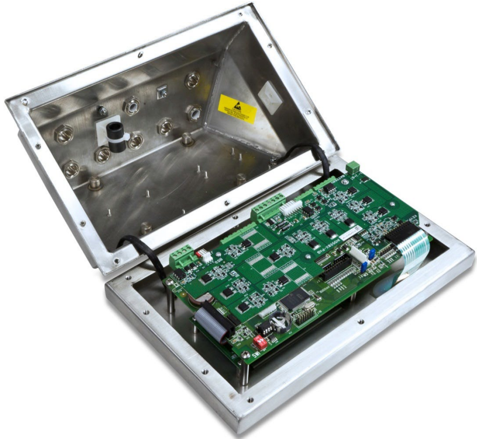
Figure 3-28: PAB Installed on IND560x Main Board
