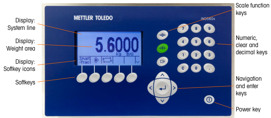
Figure 1-9: The IND560x Display and Keyboard Layout
