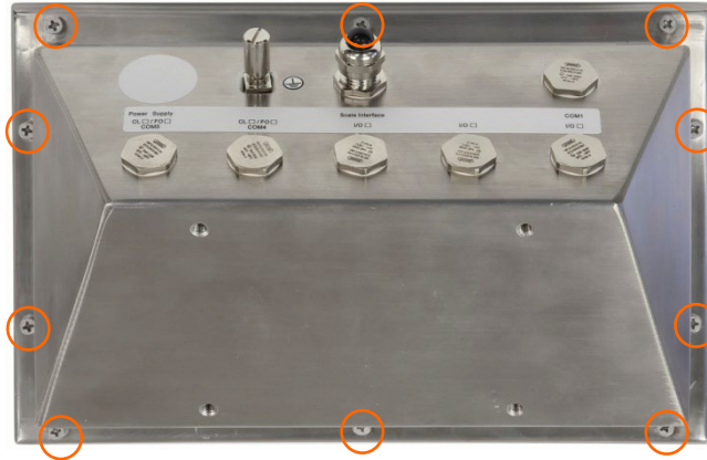
Figura 3-3: Parafusos do painel frontal
