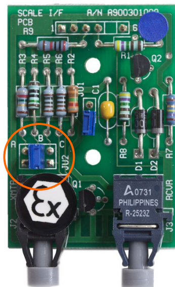
Figure 3-43: J2 Pin Location on Puma/ID3sTx FO Option PCB
