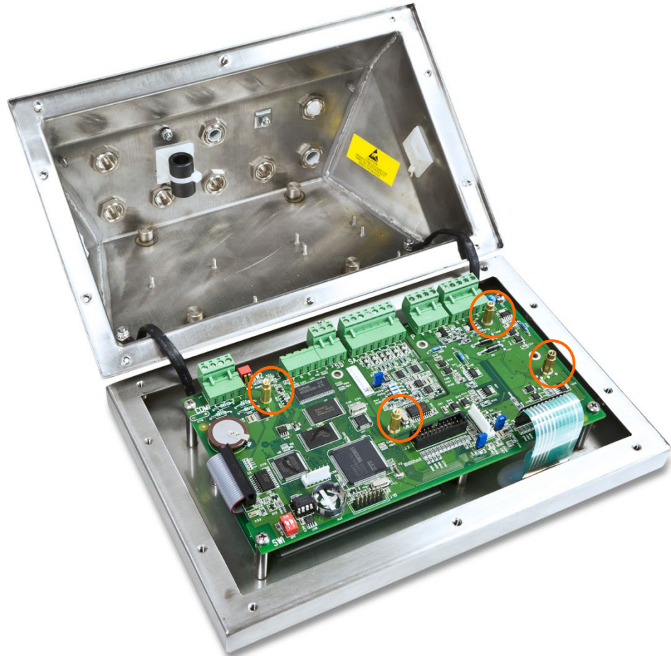
Figure 3-27: Location of IND560x-PAB Brass Standoffs
