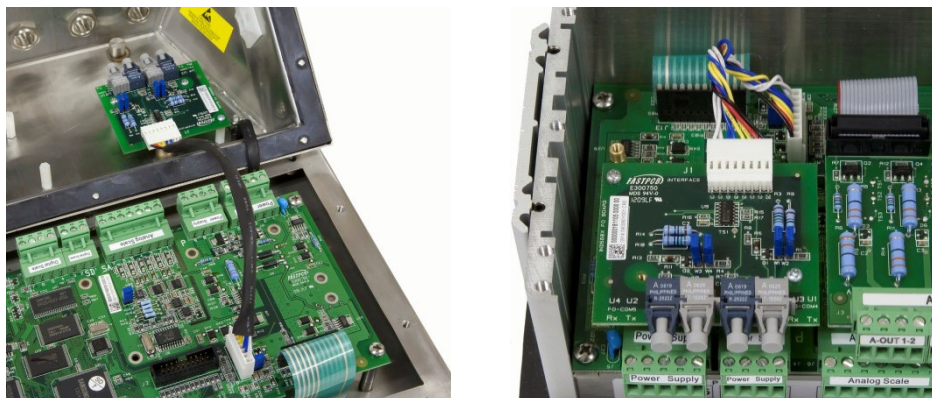
Figure 3-42: Fiber Optic Interface Board
