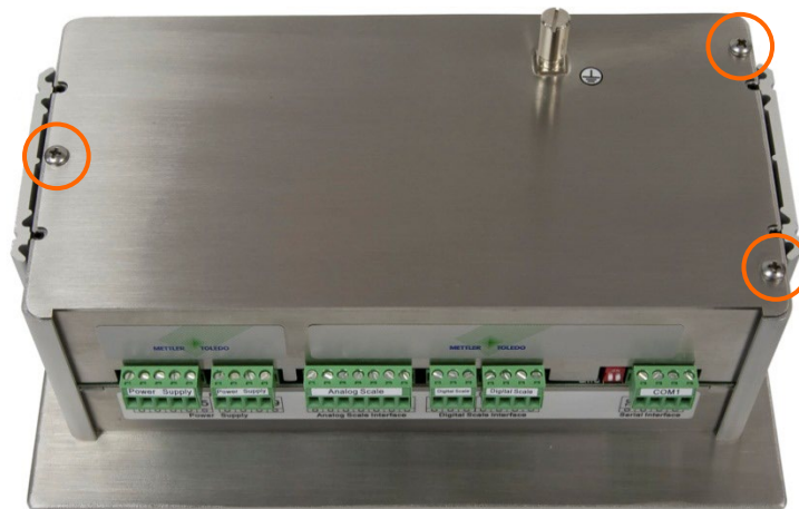
Figure 3-2: Opening the Panel-Mount Enclosure
