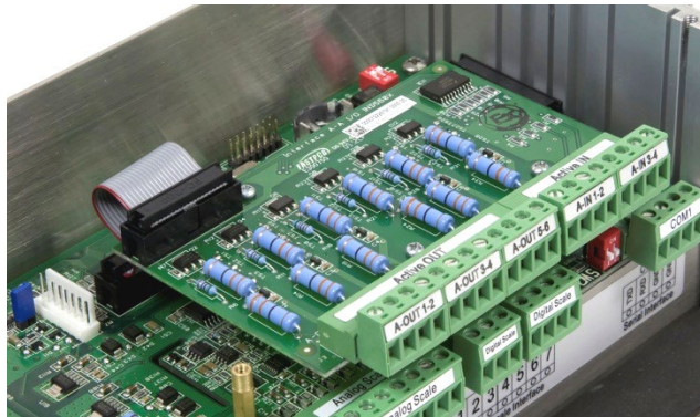
Figure 3-36: Panel-mount Enclosure Discrete I/O Installation
