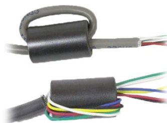
Figure A-24: Installing the Ferrite Cores
