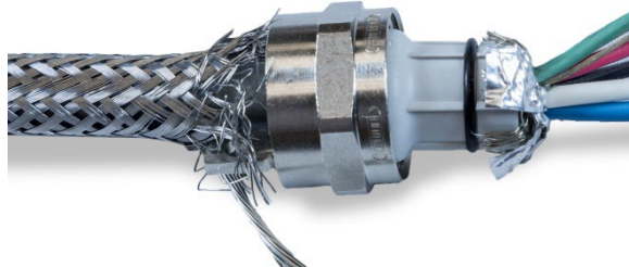
Figure A-54: Inner Braided Shield Wires and Foil Trimmed to Length and Folded Back Over Grommet
