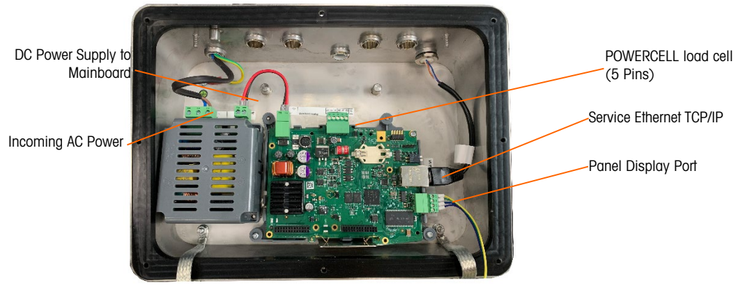
Figure A-36: POWERCELL Main Board in Harsh Enclosure
