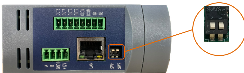
Figure 4-20: Metrology Switch Location
