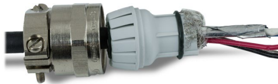
Figure A-65: Inner Shield Unbraided and Folded Back over Grommet
